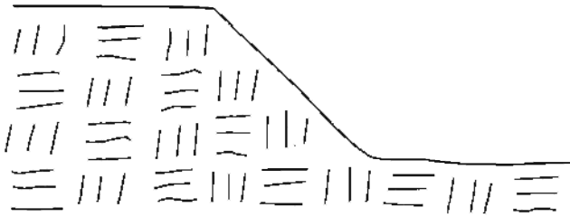
Fig. 2.7: If you've got poor drainage, it's probably a good idea to read Chapter 7 now. If you've got a shallow "angle of repose," really horrendous drainage, such as soil probably indicative of loose sandy subsoil, test reveals water table three feet down, you'd better rethink your plans altogether. Maybe you can berm a house built much nearer the surface or switch to an earth-roofed above-grade home. Underground housing does not suit every site.
